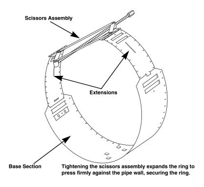
Figure 2-22 Scissors Ring adjustment
